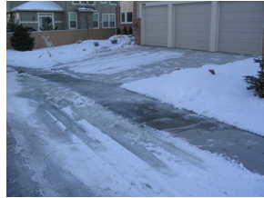
Ice is more prominent on the north side of the house or where shadows do not allow for solar melting
